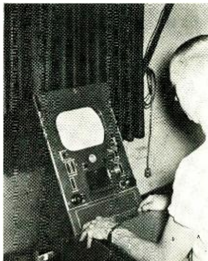
Fig. 8. Film-chain monitors must be checked regularly for picture quality.
